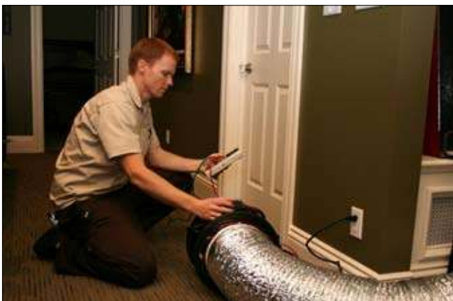
EA68 Duct Blaster Test Setup
